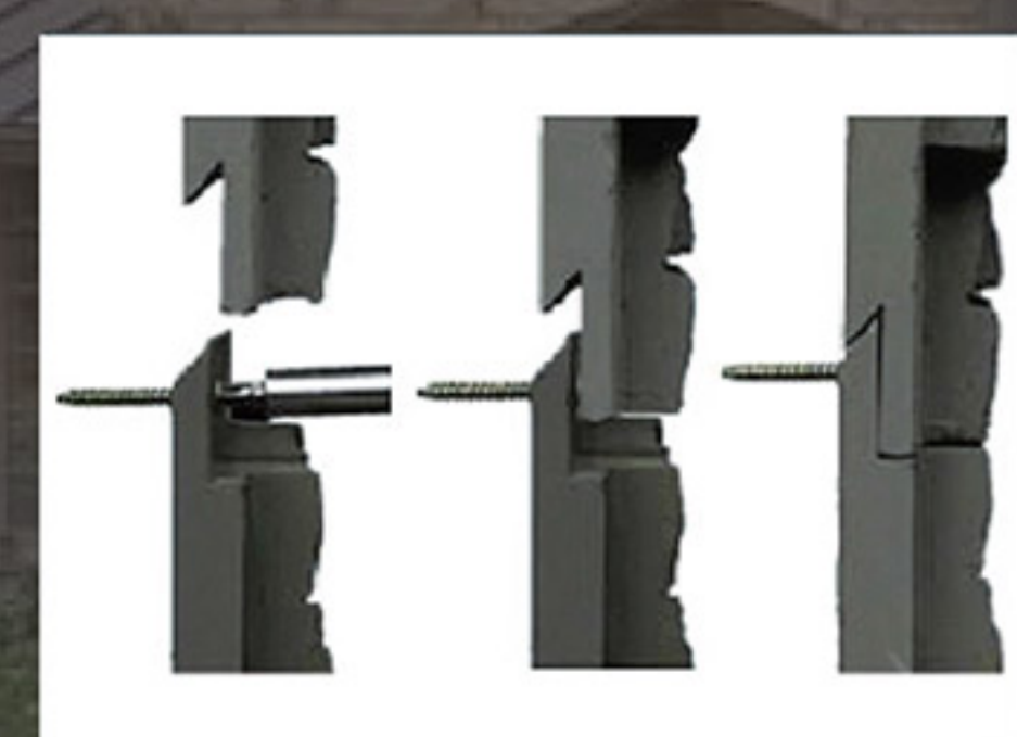
9. Upper panel interlocks with lower panel. screws are invisible.
